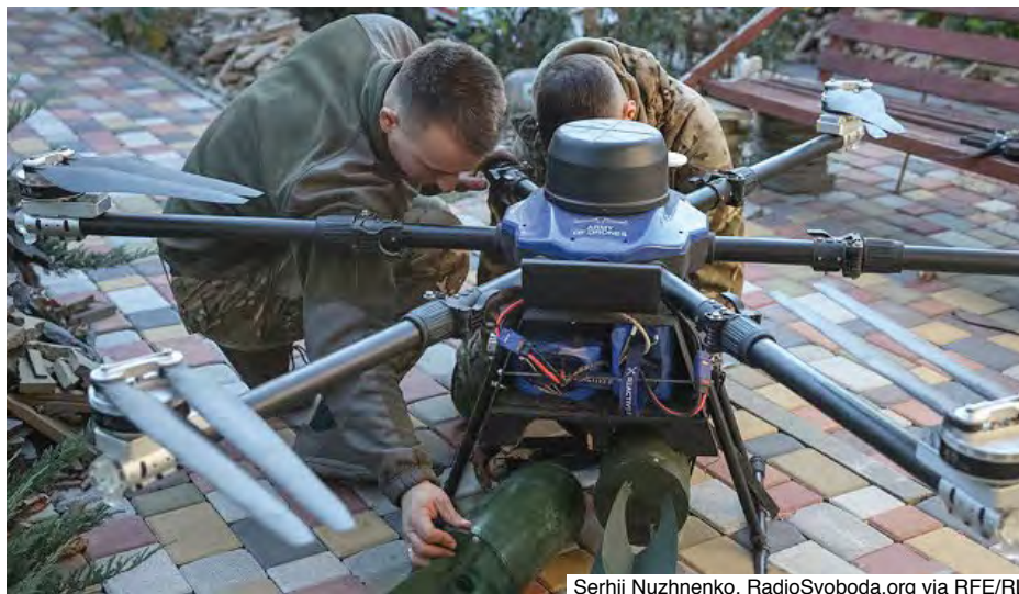
Ukrainian servicemen attach munitions to a modified drone.
