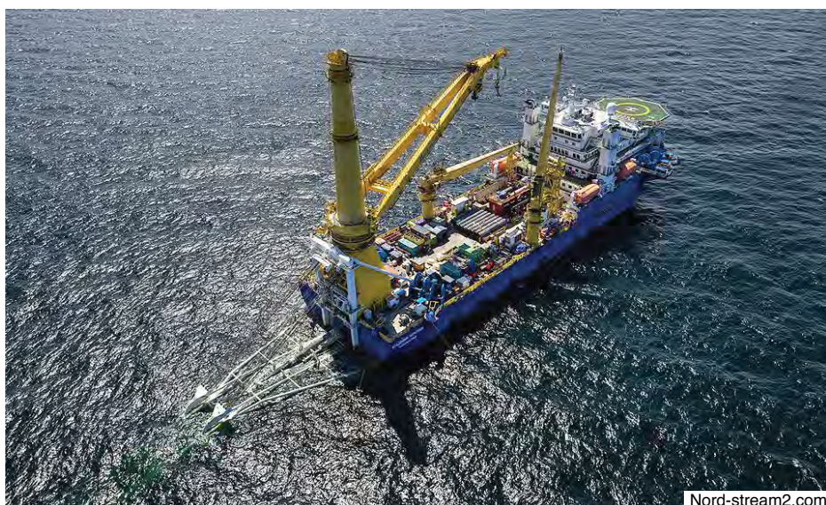
Russian pipelay vessel Akademik Cherskiy at work on the remaining section of the Nord Stream 2 pipeline in sunny German waters as seen in a photo taken in June.
